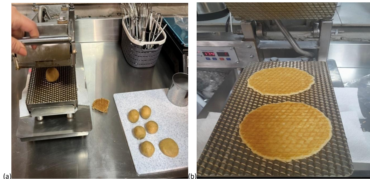
Figure 3: An experimental model of a Dutch waffle machine: The baking process (a), baked sample (b).
