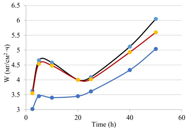
**Figure 2.** Moisture absorption capacity of Z/GM films: – Z/GM=1.5; – Z/GM/PPhC, – Z/GM/SEO.
