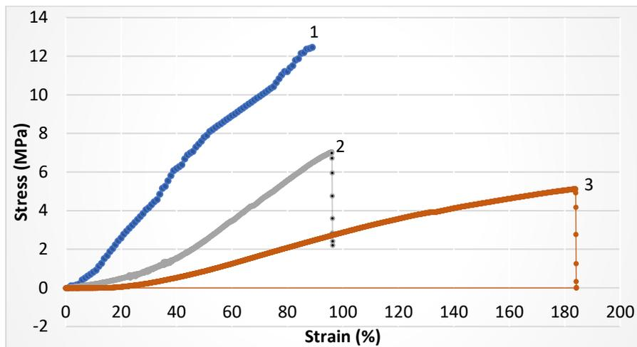
**Figure 3,** Stress-strain curves of selected Z/GM films: **1** – Z/GM, **2** – Z/GM (PPhC), **3** – Z/GM (SEO)
