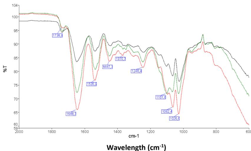
**Figure 1.** FT-IR spectra of a composite film containing EO and PPhC: — Z/GM 1.5; — Z/GM 1.5+SEO; — Z/GM 1.5+PPhC (2000-600  $\text{cm}^{-1}$ ).
